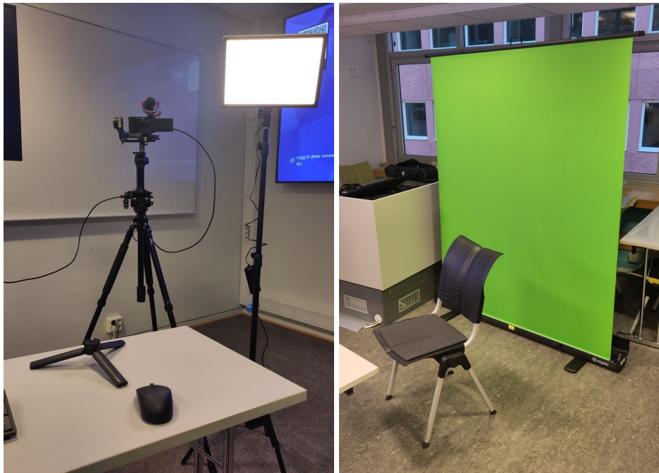
Figure 52 – Tripod with gimbal mounted camera for remote operation and green screen for background control.
